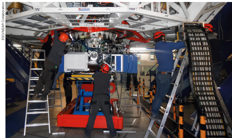
The NEAR experiment being mounted on the Cassegrain focus of the VLT's UT4 (Yepun).
